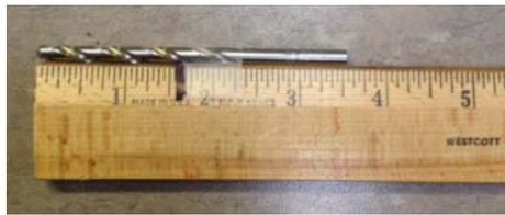
5. Use the 5/32" drill bit to initially enlarge the port. Do not exceed the depth of 1 ½". **Ensure the drill is straight, on the lowest speed and follows the existing hole.** See picture below. Do not skip this step. Starting with the 3/16" drill bit may damage the pressure port beyond repair.
